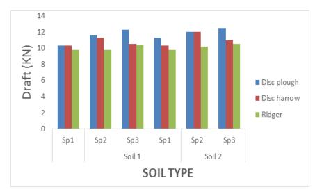
Figure 3. Effect of different forward speeds and soil on implementing draft force (KN) at the different soils
