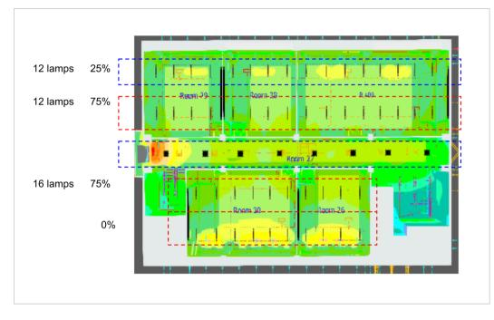
Fig. 10 Grouping and dimming after improved daylighting
