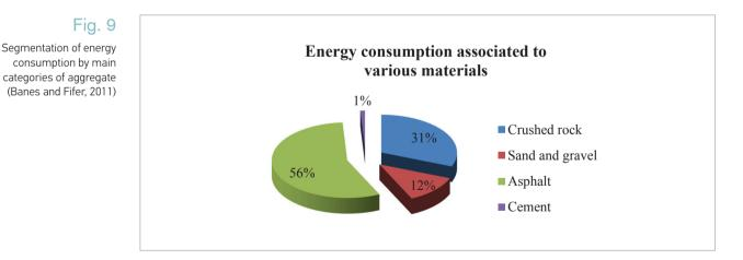
However, these amounts may decrease considerably if the aggregates excess water is reduced as the highest proportion of energy is consumed for drying and heating the aggregates. Another way the improvement the manufacturing process involves the use of recycled asphalt mixtures, resulting in reductions of up to 50% of emissions (Andrei, et al., 2014).
