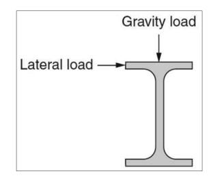
Figure 2: Lateral load applied on the upper flange
