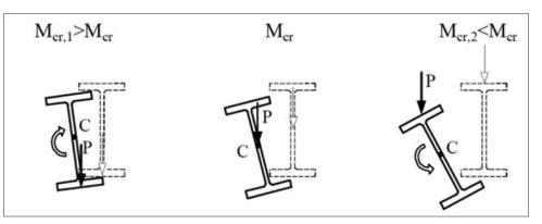
Figure 5: The influence of the level of the applied load on the capacity of the section
