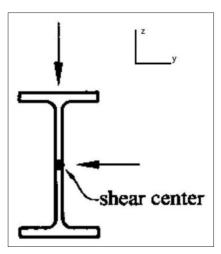
Figure 1: Pure biaxial bending<sup>[2]</sup>
