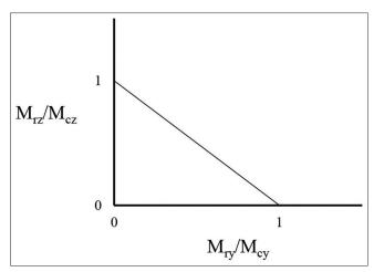
Figure 3: Simple linear interaction for biaxial bending<sup>[2]</sup>
