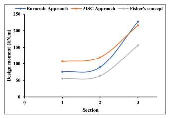
**Figure 8:** Comparison between the three approaches for design moment about Z-axis
