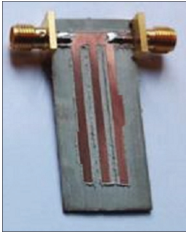
Figure 10: Actual implementation of the matching circuit
