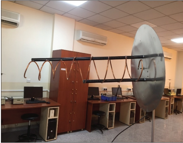
Figure 6: Non-uniform helical antenna manufactured
