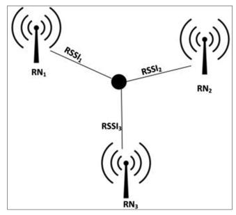
Figure 1: Received signal strength indicator based positioning<sup>[11]</sup>
