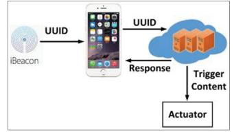
AQ1 Figure 4: Model architecture for iBeacon systems<sup>[28]</sup>
