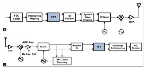
AQ1 Figure 2: Orthogonal frequency division multiplexing (a) transmitter and (b) receiver block diagram<sup>[9]</sup>
