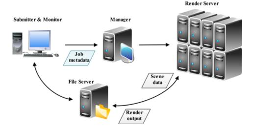
Figure 1 Architecture of the Distributed Rendering System
