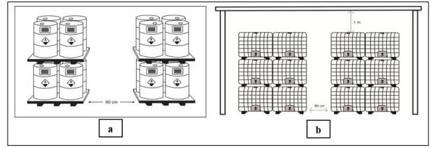
Figure 4. Rack placement on Hazardous Waste Station (a) for Drum and (b) for Wooden Boxes [21]
