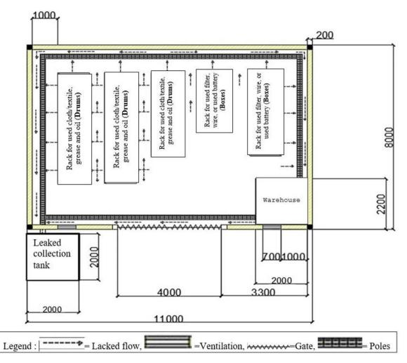
Figure 5. Top View of Hazardous Waste Station in XYZ Port Area
