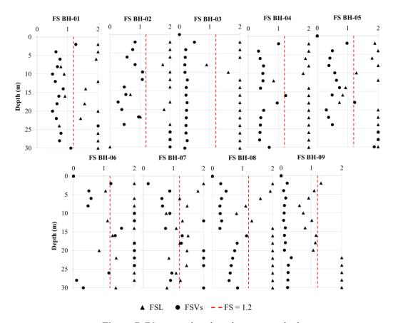
**Figure 7.** FS comparison based on two methods.
