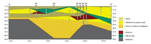
**Figure 4.** Soil stratigraphy of cross-section A-A'.
