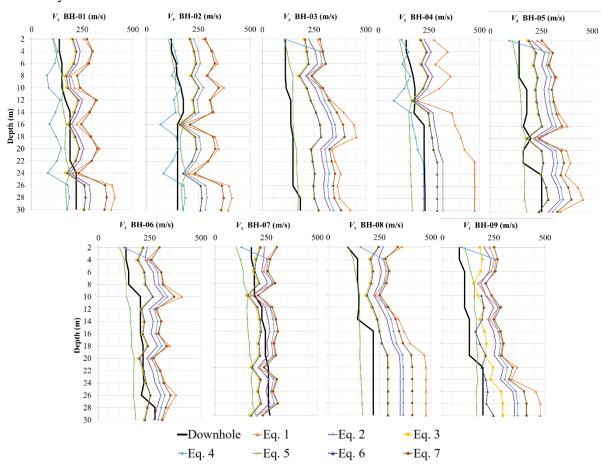
**Figure 6.** N-SPT and  $V_s$  correlation based on given equations.
