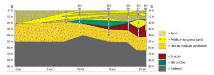
Figure 5. Soil stratigraphy of cross-section B-B'.
