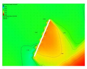
Figure 10. Distribution of wave height in surround breakwater due to  $H_s = 4.0$ m.
