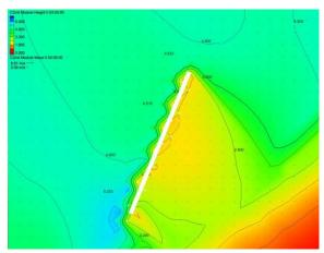
Figure 12. Distribution of wave height in surround breakwater due to  $H_s = 5.0$ m.
