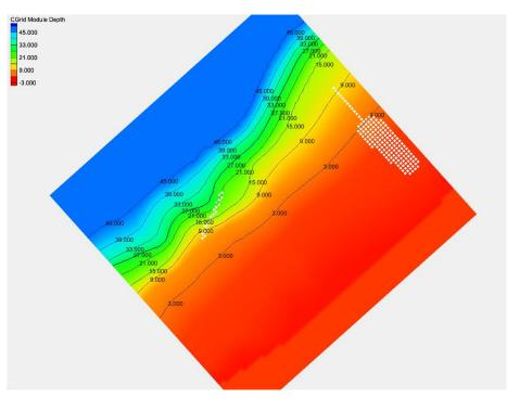
Figure 7. Numerical model bathymetry grid for 2D wave model of Waikelo Port
