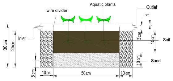
Figure 1. Modeling design of constructed wetland (side view).
