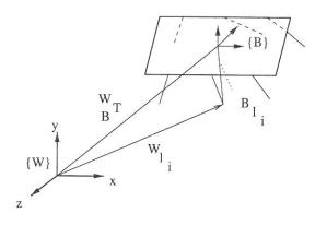
*Fig. 2.* A schematic showing world frame and body frame.
