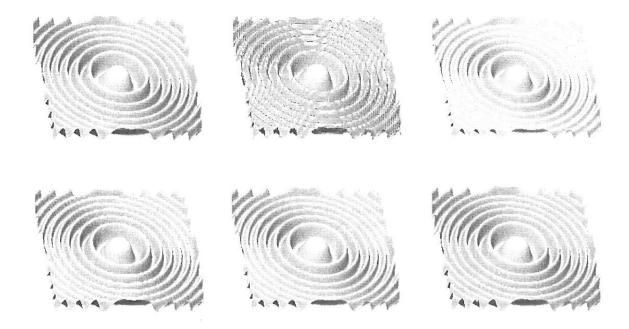
*Fig.* 6. Six different reconstruction methods in 3D. a) reconstruction with sinc function, b) nearest neighbor, c) 3-rd order B-spline approximation, d) linear interpolation, e) Mitchell reconstruction with B = C = 1/3 and f) 3-rd order B-spline interpolation.
