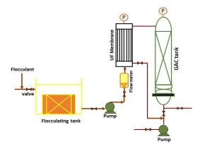
Figure 7 Schematic diagram of system setup.
