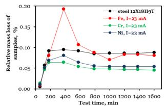
**Figure 3** The nature of the change in the relative mass loss of samples obtained by non-vacuum electron beam surfacing of amorphous boron with various wetting components, from the time of exposure to nitric acid. Surfacing current is 23 mA.
