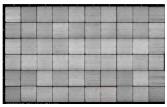
**Fig. 2** Photo of the electroluminescence of the module at the end of the thermal cycling tests
