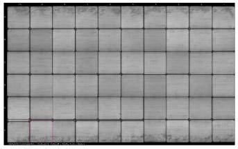
Fig. 1 Photo of the electroluminescence of the module at the end of the tests
