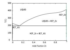
Fig. 3. Calculated Sn-Zn phase diagram
