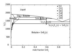
Fig. 13. The calculated In<sub>2</sub>O<sub>3</sub>-SnO<sub>2</sub> phase diagram in air compared with experimental data [1, 18–21, 42]
