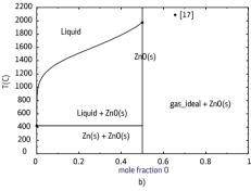
Fig. 8. Calculated Zn–O phase diagram: *a* — with participation of the gas phase, *b* — without
