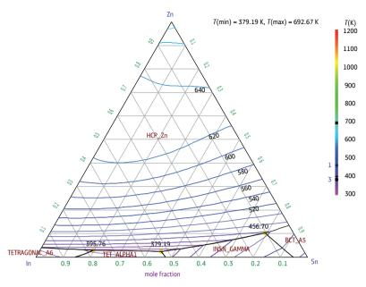
Fig. 4. Calculated liquidus surface in the In-Sn-Zn system
