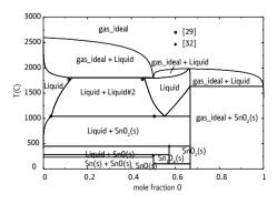
Fig. 7. Calculated Sn-O phase diagram compared with experimental data [29, 32]
