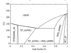
Fig. 1. Calculated In-Sn phase diagram
