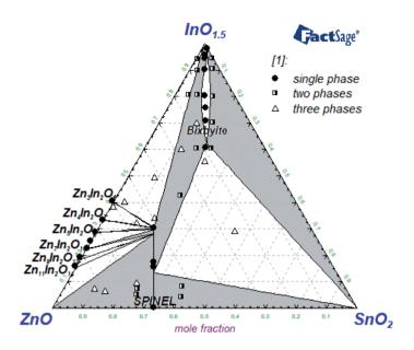
Fig. 18. Subsolidus phase relationships in  $In_2O_3$ -SnO $_2$ -ZnO system in air at 1275 °C and 1 atm compared with experimental data [1]. Grey areas are the two-phase regions
