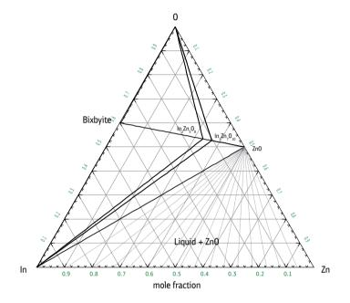
Fig. 11. The calculated In-Zn-O isothermal section at 500 °C
