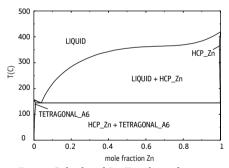
Fig. 2. Calculated In-Zn phase diagram
