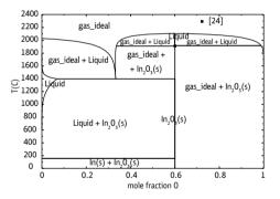
Fig. 5. Calculated In-O phase diagram
