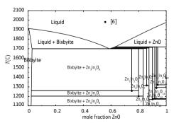
Fig. 15. The calculated In<sub>2</sub>O<sub>3</sub>–ZnO phase diagram in air compared with experimental data [6]
