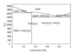
Fig. 16. Calculated SnO<sub>2</sub>–ZnO phase diagram in air
