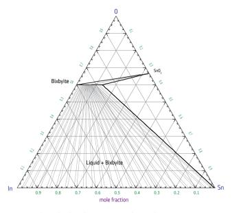
Fig. 10. The calculated In-Sn-O isothermal section at 500 °C
