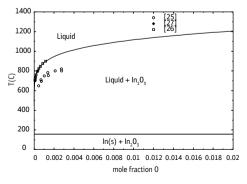
Fig. 6. Calculated phase equilibria in the In-rich part of the In-O diagram compared with experimental data [25–27]
