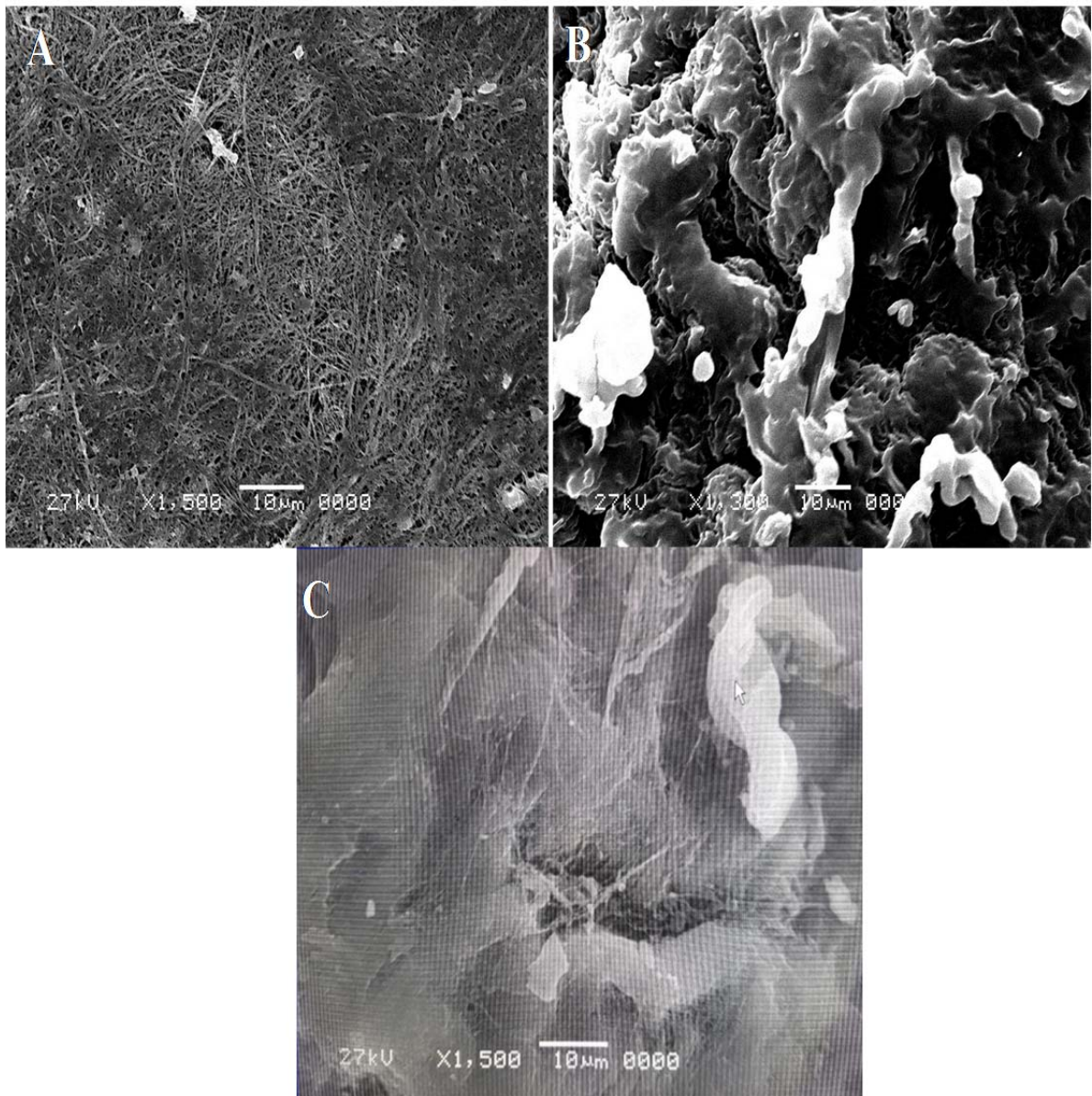
Figure 1: Scanning Electron Microscopy of the films, (A) BC, (B) PHB film and (C) blenda CB + PHB.
