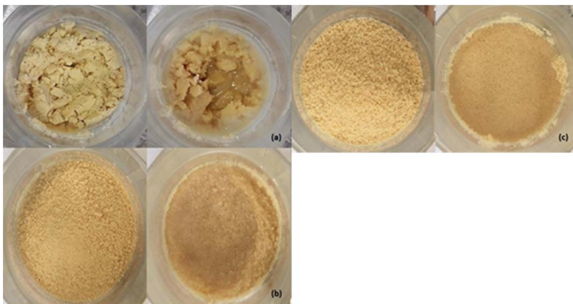
Figure 4: Wetting time tests for (a) raw PPI and (b) agglomerated test 1 and (c) agglomerated test 2.
