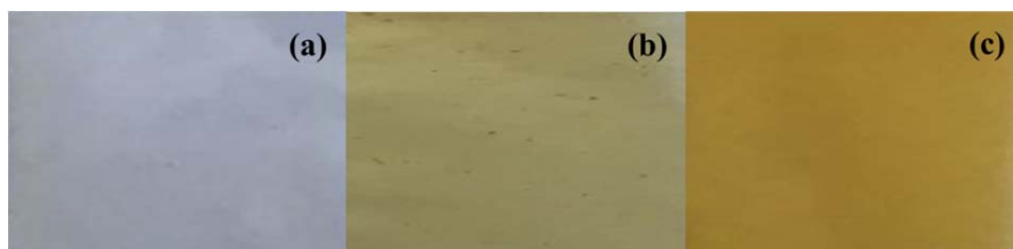
Figure 1: Film packaging appearance produced with Brazilian pine seeds starch, citric pectin and Acca sellowiana extracts; (a) FPC; (b)FPPe; (c) FPHe.
