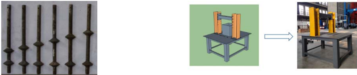
Figure 1: Small scale model pile with semi-circle section Figure 2: The platform for Loading
