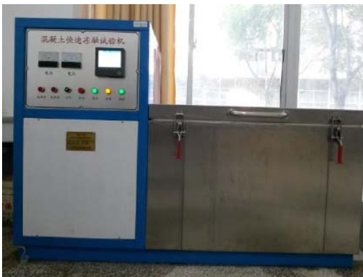
Figure 3: The testing machine TDR-28 of rapid freezing and thawing of concrete
