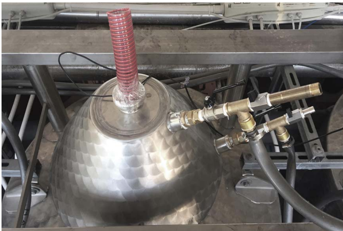
Figure 1: Condensation system above a fermentation tank.
