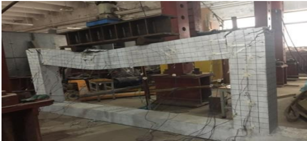
Figure 2: Failure mode of the test piece
