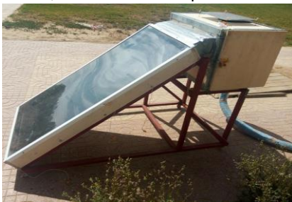
Figure 1: Experimental setup (solar collector with drying chamber) Figure 2: Holes of inlet solar collector
