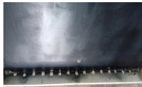
Figure 1: Experimental setup (solar collector with drying chamber) Figure 2: Holes of inlet solar collector
