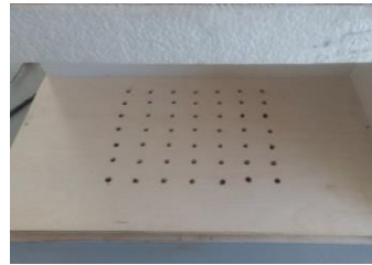
Figure 4: Orifices into drying chamber
