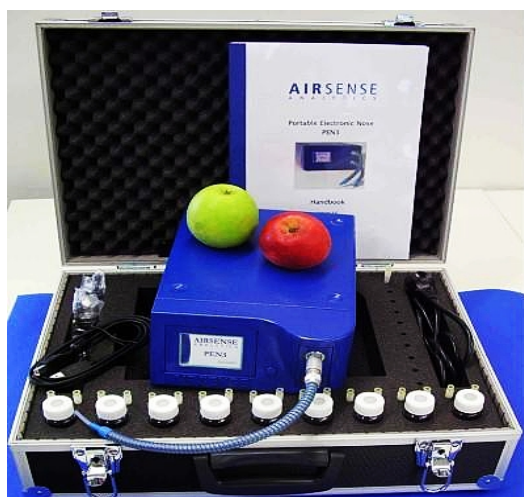
Figure 1: PEN3 electronic nose
