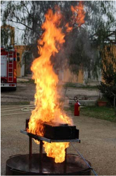
Figure 7 – A picture of the battery pack during thermal abuse test.
