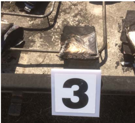
Figure 1 – A picture of the cell after thermal abuse test.
