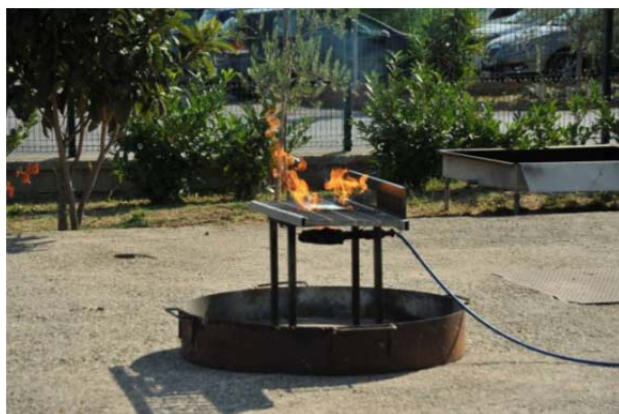
Figure 3 - Experimental setup for thermal abuse tests.
