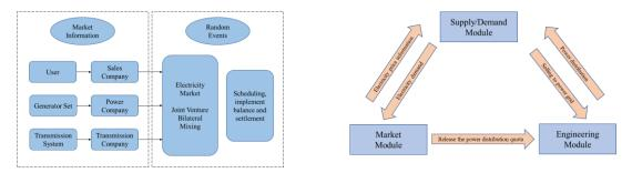
Figure 5: Basic block diagram of electricity market Figure 6: Electricity market three module diagram simulation
