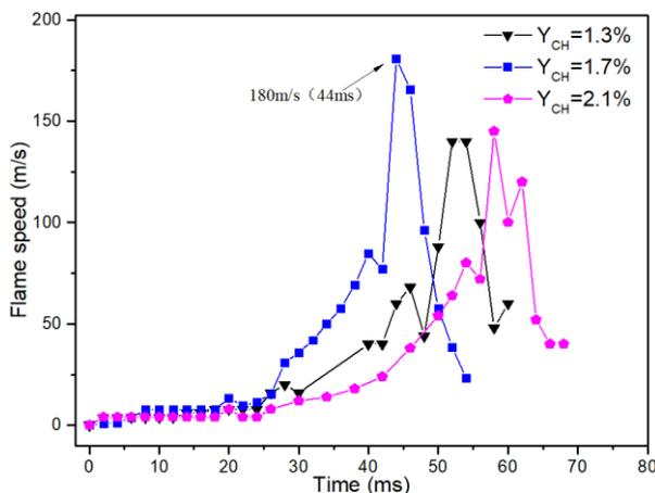
Figure 5: flame speeds along the pipe versus time
