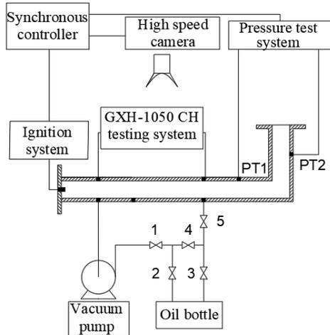
Figure 1: Schematic diagram of the explosion pipes
