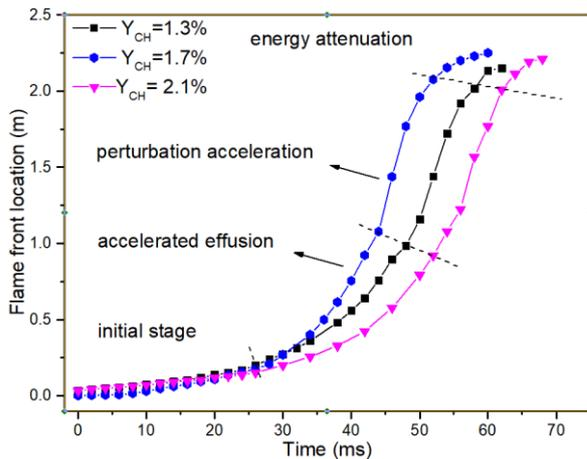
Figure 4: flame front locations along the pipe versus time
