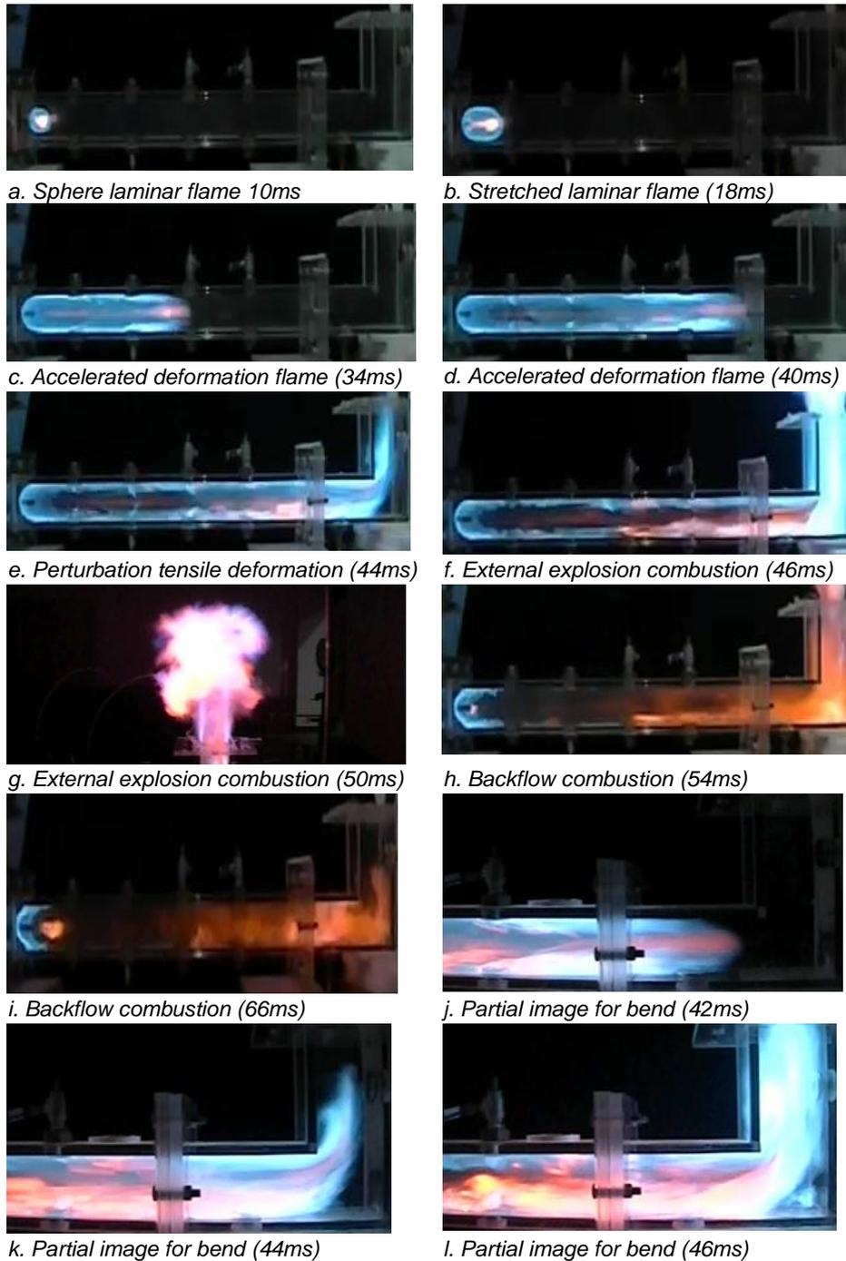
Figure 3: Flame propagation image
