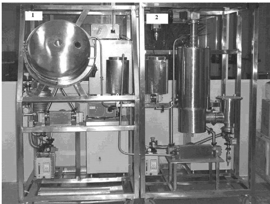
Figure 1: Developed Reactive Molecular Distillation Unit; 1 indicates the reactive molecular distiller - 2 indicates the system for removal the light compounds
