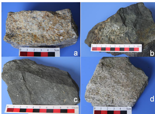
Figure 2: The main magmatic rock types of the research area (a: plagioclenite, b: andesitic porphyrite, c: tuff, d: diorite).
