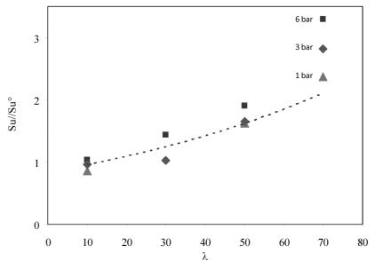
Figure 5. Ratio of the laminar burning velocity calculated from the pressure time history  $(S_u)$  to the laminar burning velocity of methane  $(S_u^O)$  versus the hydrogen content in the fuel,  $\lambda$ , at different initial pressures. The dotted line represents the  $S_u/S_u^O$  ratio as calculated by Le Chatelier's rule-like formula at 1 bar.
