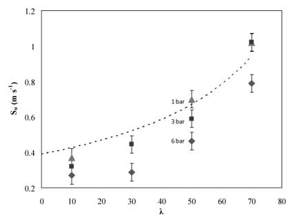
Figure 4. Laminar burning velocity  $(S_u)$  calculated from the pressure time history versus the hydrogen content in the fuel,  $\lambda$ , at different initial pressures. The dotted line represents  $S_u$  as calculated by Le Chatelier's rule-like formula at 1 bar. The data for  $\lambda = 10\%$  come from Cammarota et al. (2009).
