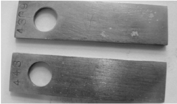
Figure 2: The steel after corrosion experiment
