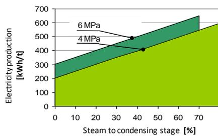
Figure 2: Specific electricity production
