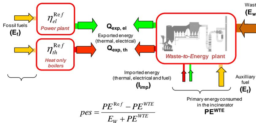
Figure 4: Graphical representation of Primary energy savings criterion
