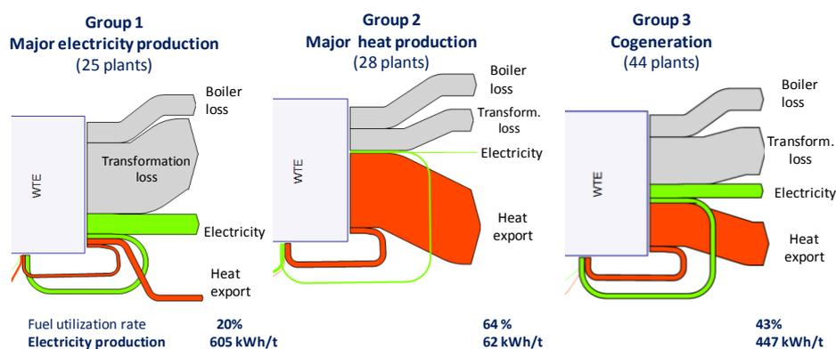
Figure 1: Classification of facilities and obtained efficiency (97 facilities associated in CEWEP, Reimann 2006)
