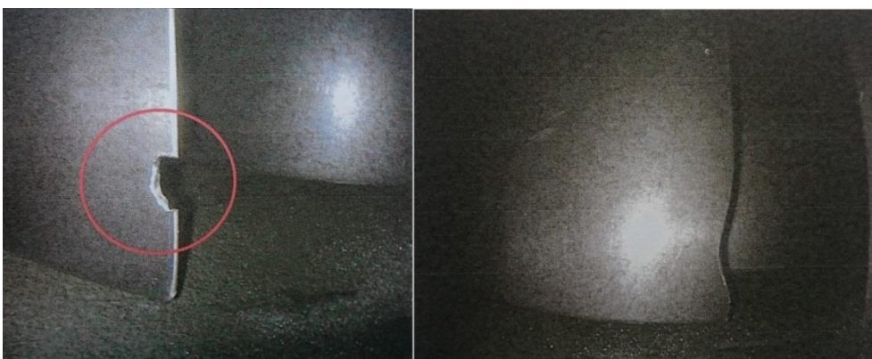
Figure 3: Compressor blade before and after repair (grinding)
