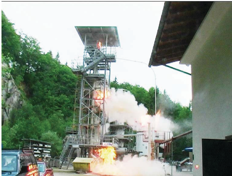
Figure 4: Examples of the vented dust explosion in the bucket elevators - K_{St} \leq 150 bar·m·s -1
