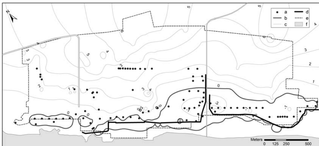
Figure 1: Piezometric map (equidistance 1 m) of the study area; a) pumping wells; b) piezometric line 0 m a.s.l.; c) piezometric lines; d) physical barrier; e) Refinery boundary; f) sea.
