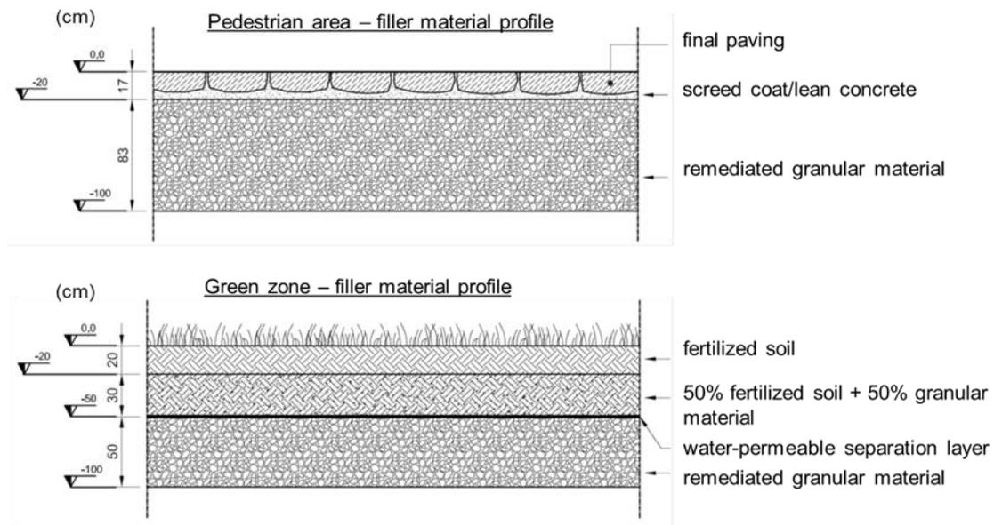
Figure 1: Filler material sections
