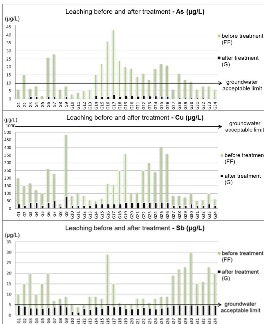
Figure 2: Comparison of As, Cu and Sb concentrations in the leachate before and after treatment.
