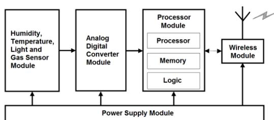
Figure 6: Block Diagram of the sensor nodes.
