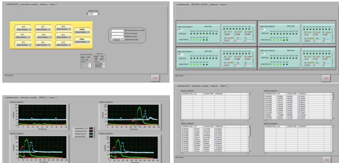
Figure 5: Front panel of the control program: a) Configuration, b) Masks and values, c) Graphs and d) Tables.
