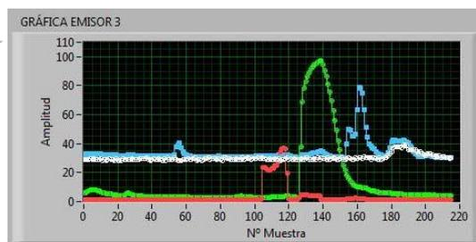
Figure 7: Measurements of one of the sensor nodes: Temperature (white), Light (Red), Air Quality (green) and Humidity (Cyan).
