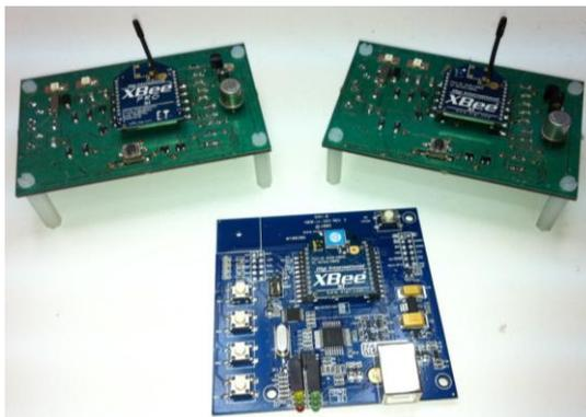
Figure 3: Image of the nodes and host of the network.
