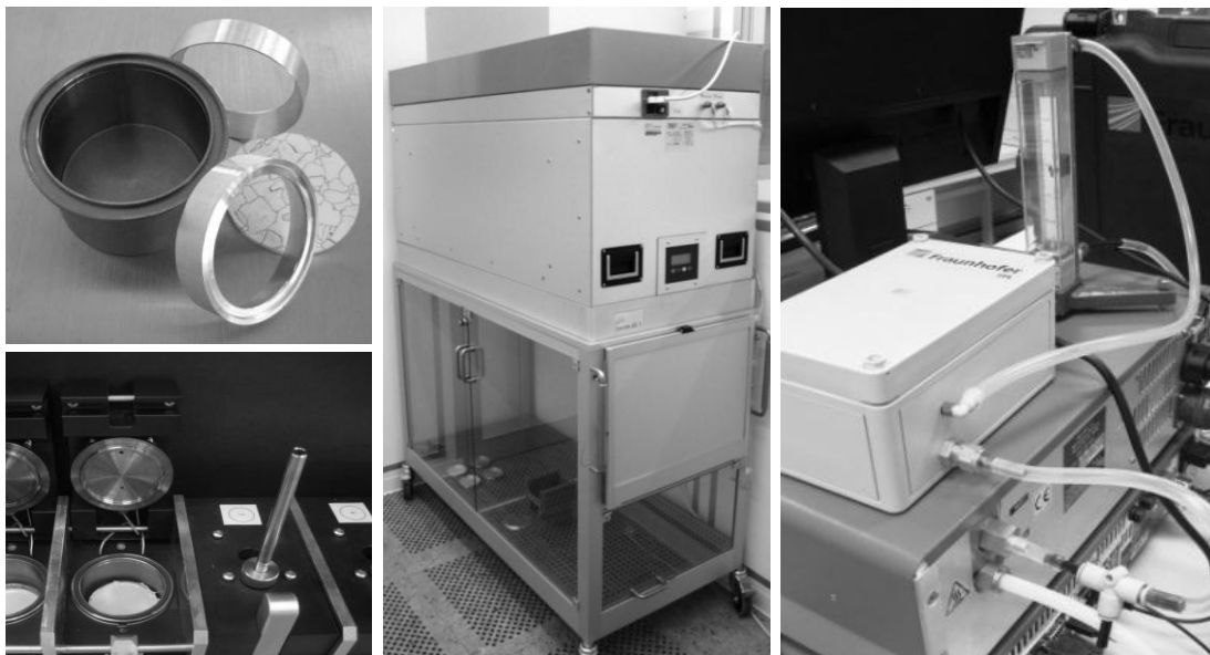
Figure 1: Upper left: Representative material sample with a sampling chamber and overlying ring for determining the surface-specific emission rate of the material sample. Lower left: Material samples in micro-chamber with one cover lid opened and other lid closed with an adsorption tube attached on the outlet of the closed chamber. Middle: storage environment with VOC filtration. Right: setup for experimental prove of the calculation model
