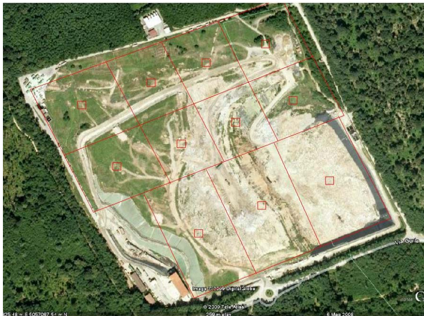
Figure 2: Division in sub-areas of the landfill surface
