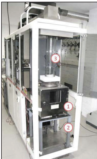
Figure 1 : Modified Cone Calorimeter with combustion chamber (1), lowered stand framework (2) and chimney (3)
