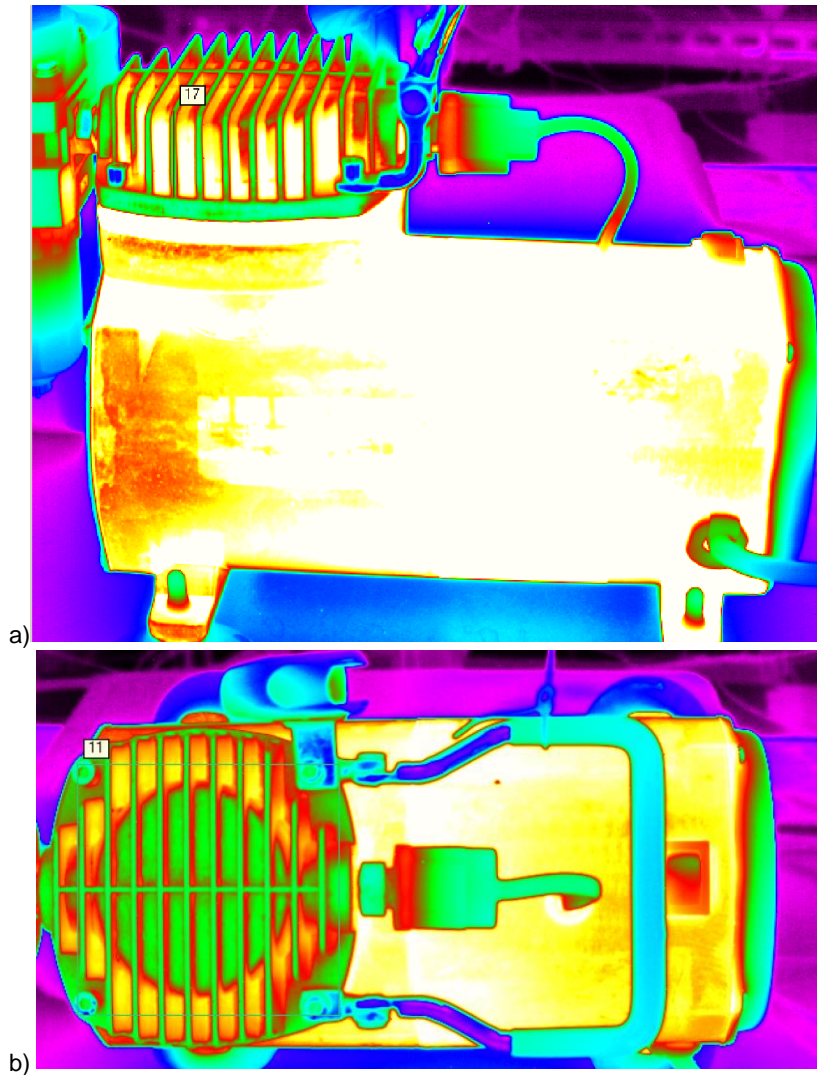
Figure 2: Thermogram of the compressor: a) side view b) upper view
