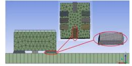
Figure 3: Finite element model of ADXL78
