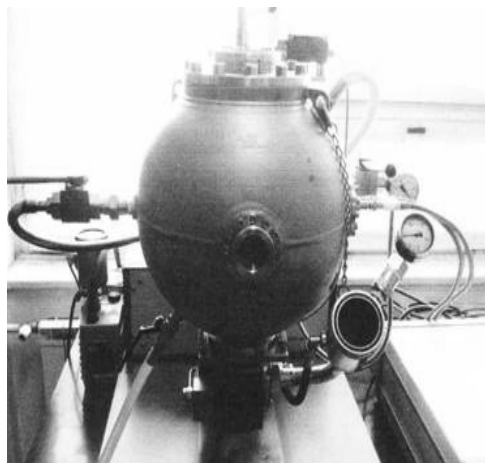
Figure 2. Investigation device for determination of powder explosion characteristics
