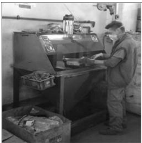
Figure 1. Device for recycling of waste toner cartridges
