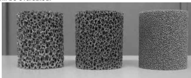
Figure 3: SiC-made ceramic open foam samples for catalyst support
