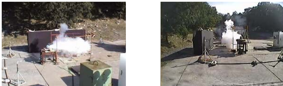
Figure 4: Release of LPG
