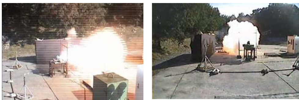
Figure 6: Ignition of LPG cloud
