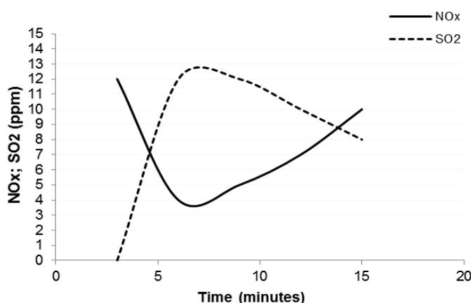
Figure 4: NO<sub>x</sub> and SO<sub>2</sub> levels released during the briquettes combustion.
