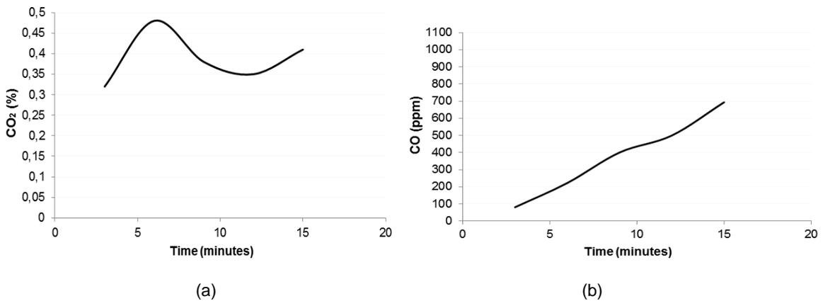
Figure 3: CO<sub>2</sub> (a) and CO (b) levels released during the briquettes combustion.
