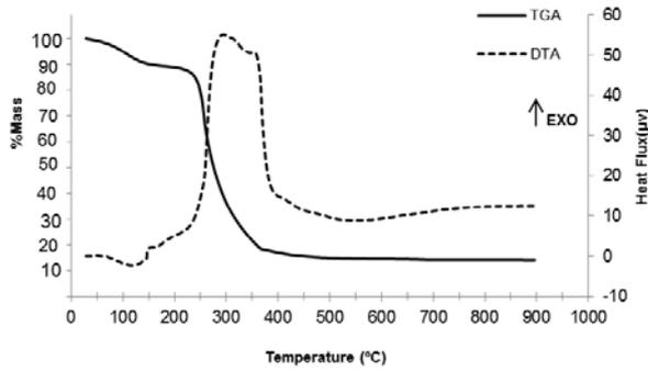
Figure 1: TGA and DTA for banana leaves briquettes.
