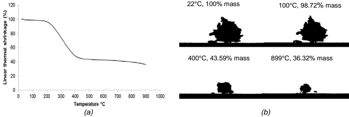
Figure 2: Linear thermal shrinkage curve (a) and images of mass degradation (b) for banana leaves briquettes.
