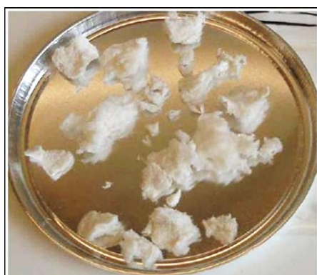
Figure 1(a) (Left): Macroscopic image of the pure cellulose after three step treatment. 1(b) (Right): SEM image of the pure cellulose after treatment.
